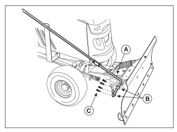
Figure 16. Control Arm Removal
